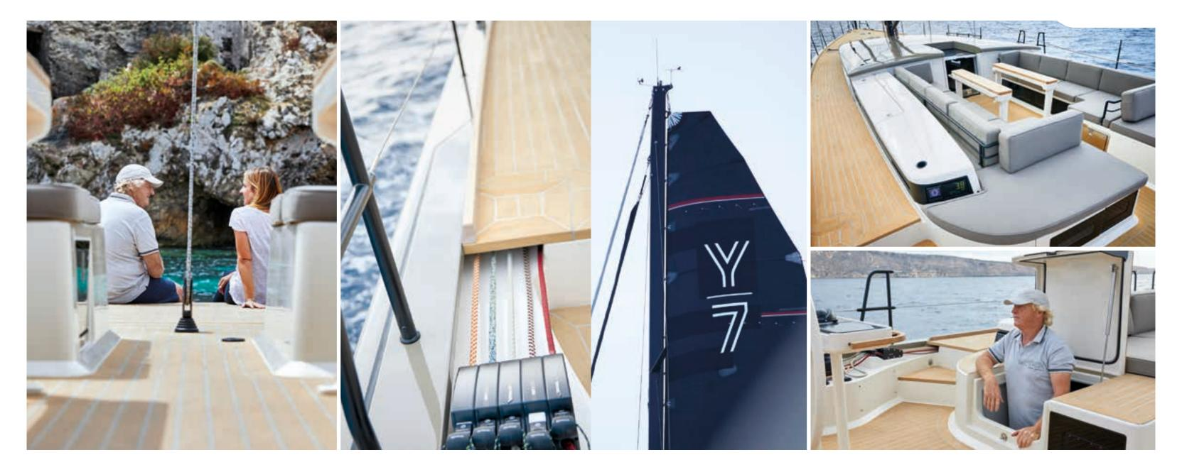
All halyards and sheets on the Y7 run hidden to the helmstation. The helmsman operates the Y7 himself – probably the only 70 footer on the market. As there is no backstay, the square headed mainsail has a better profile and more sail area. The cockpit has a high variety of uses. On the portside there is a full size companionway into the crew quarters invisibly integrated in the aft cockpit settees.
